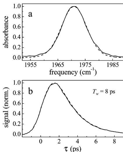
**Figure 4.** (a) Experimental linear spectrum and (b) vibrational echo decay data at  $T_w = 8$  ps (solid lines) overlaid with the best-fit linear spectrum and vibrational echo decay ( $T_w = 8$  ps) calculated from nonlinear response theory (dashed lines) for H64V in trehalose at  $1971\text{ cm}^{-1}$ .
