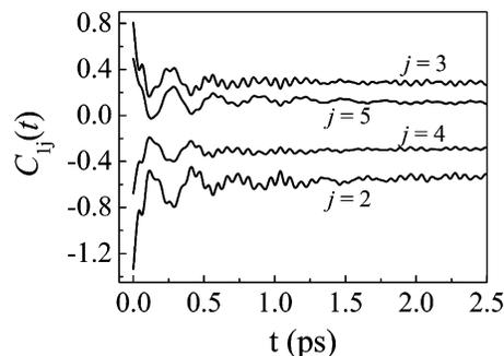
**Figure 9.**  $C_{ij}(t)$  (rad/ps)<sup>2</sup>, the cross-correlation functions of the contributions to the fluctuating CO frequency of protein shell 1 (outermost) and shells  $j = 2, 3, 4,$  and  $5$ , as calculated from MD simulations of H64V in dynamic water solvent.
