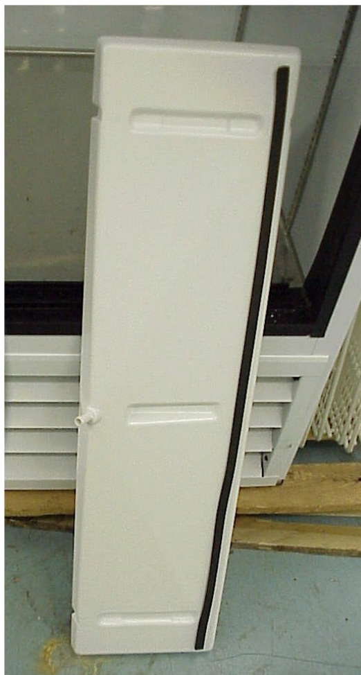
Evaporator pan -must also be removed to access evaporator coils.
