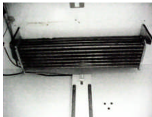
Figure 6. Evaporator pan, drain tube, and temperature sensor.
