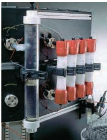
Fig 11.14. A 60 ml sample volume can be run on four HiPrep 26/10 Desalting columns connected in series.
