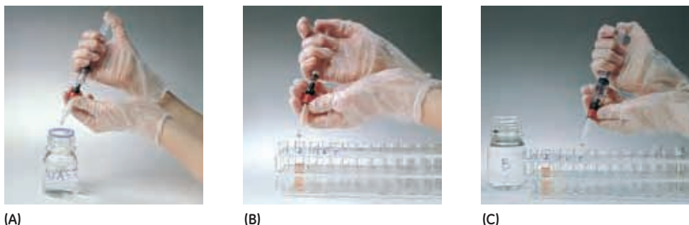
Fig 5.9. Using a GSTRap column with a syringe. A) Prepare buffers and sample. Remove the column's top cap and snap off the end. B) Load the sample and begin collecting fractions. C) Wash and elute, continuing to collect fractions.
