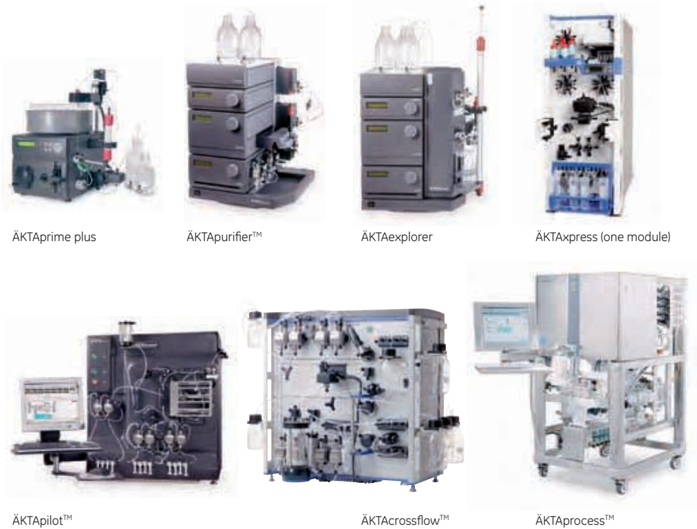
Fig 2.4. The standard ÄKTAdesign configurations.
